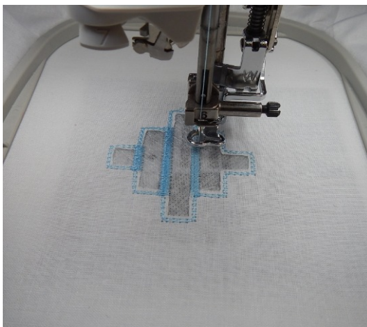
3. Remount the hoop and let the machine finish the bridges crossing the open area and the satin around the shape
