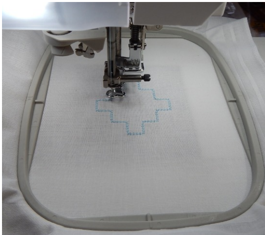
1. Stitch the first layers: the boundary around the cut area
