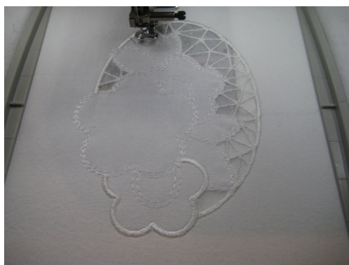
Bridges are sewn next, followed by the rest of the design. For this finishing satin I used the same Special Satin, but changed Width into 3.5 and Spacing into 0.6.
